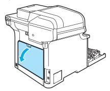
4 Pull down the two green levers, one on the left-hand-side and one on the right-hand-side, as shown in the illustration below, and then fold down the fuser cover (1).
